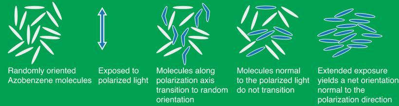
non-mechanical alternative. Photoalignment materials work through many mechanisms: photochemical crosslinking, photodegradation of polyimides, and through the reversible *cis-trans* photoisomerization
