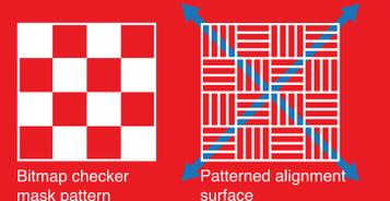
alignment direction for the two stable configurations, homogeneous planar and twisted planar, for which switching occurs via orthogonal in-plane electric fields. The maskless photoalignment method can further be used to fabricate flexible bistable displays which are attractive due to their low-power consumption, low cost, and ease of manufacturing.
